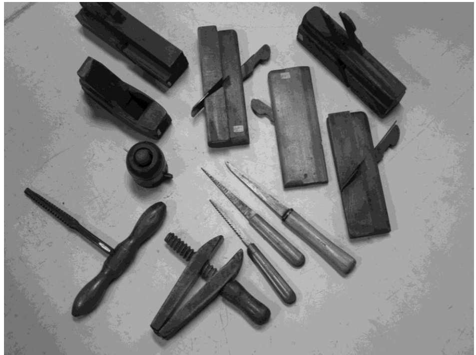
ABOVE: A molding plane, signed by Wat Thomas, designed to make sculpted molding.
